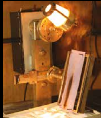
Image of Protal fabric passing EN 11612-E (Iron splash)
